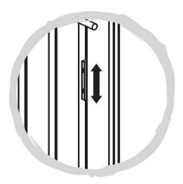
2. Place the hooks, then use hook screws through washers and holes of the hook, screw into the sliding block on the radiator, tighten the screws with the wrench.
